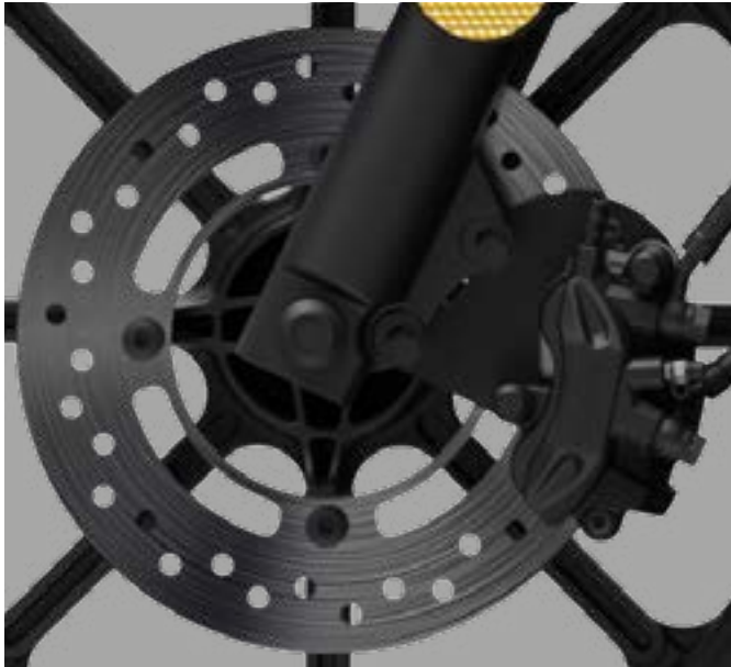
Front disc brake ø240mm
