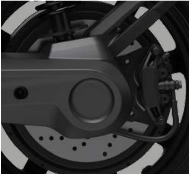
Rear disc brake ø180mm
