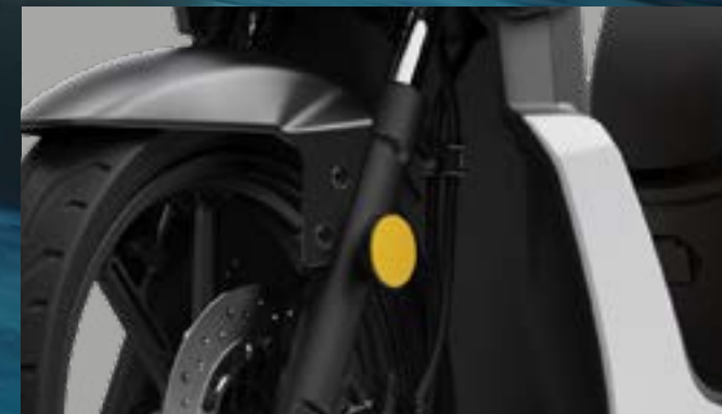
Front suspension ø31.5mm
