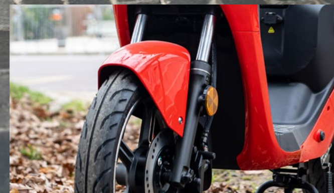
Front suspension ø26mm
