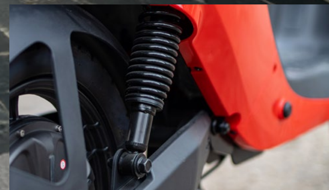
Rear suspension ø25mm
