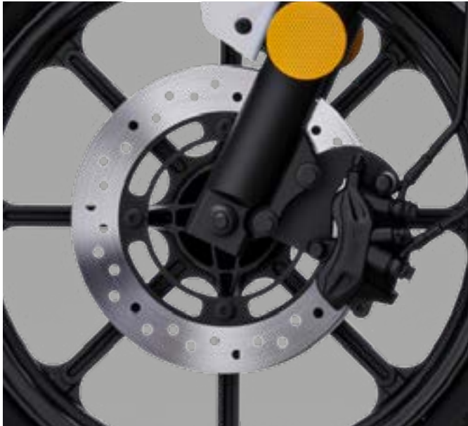
Front disc brake Ø240mm
