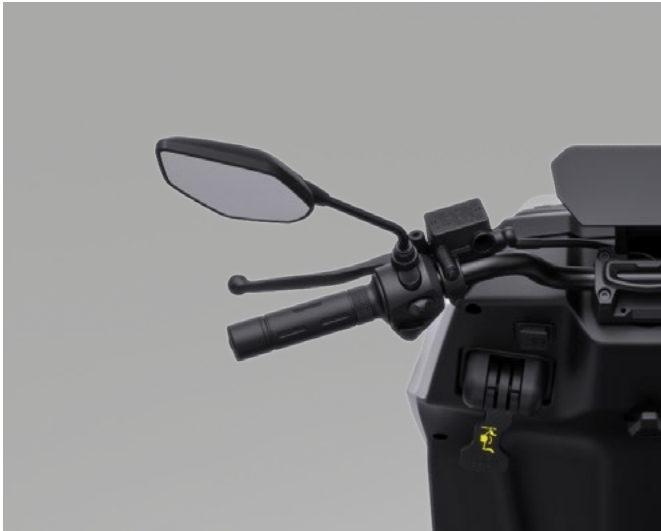
Left handlebar Rear brake.
