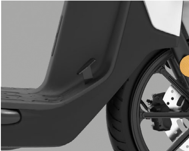
Foot brake The foot brake ensures combined braking.
