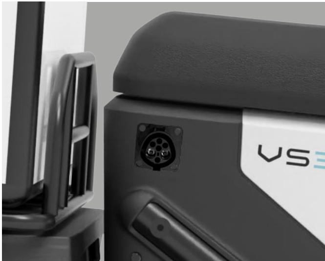
Optional Type 6 fast charging. 30 min with 13.2 kW; 35 min with 6.6 kW.
