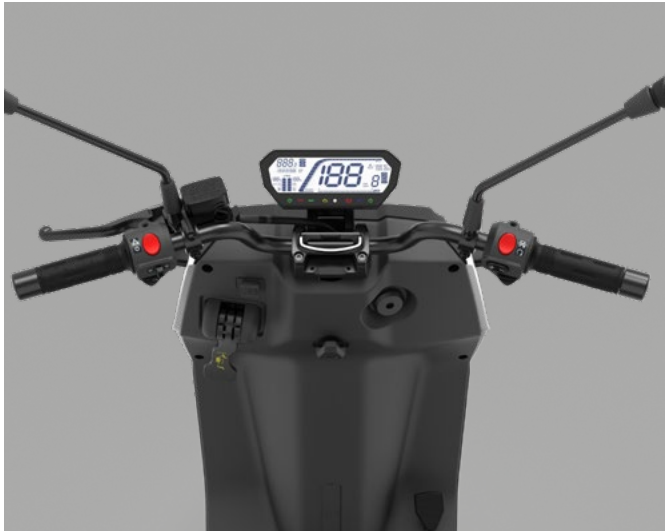
Handlebar No brake on right side. Rear brake on left side.
